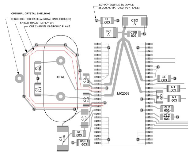
Components are identified by function (top line) and by typical package type (bottom line) which may vary.
